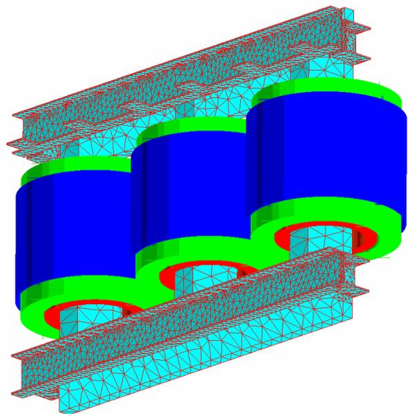
Fig.1. 3-D Finite element model of power transformer.
