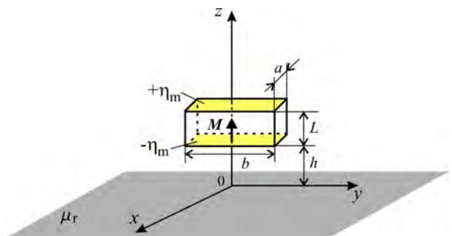
Fig.2. Permanent magnet and infinite linear magnetic plane.
