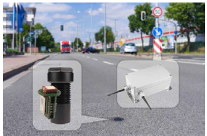
Fig. 1. Actual installation of a detector (electronics and housing shown separately) at an intersection in Erfurt. The position of the detector in the road can be recognized by the dark patch on the street. The gateway is attached to a traffic lights post at a height of 4 m.
